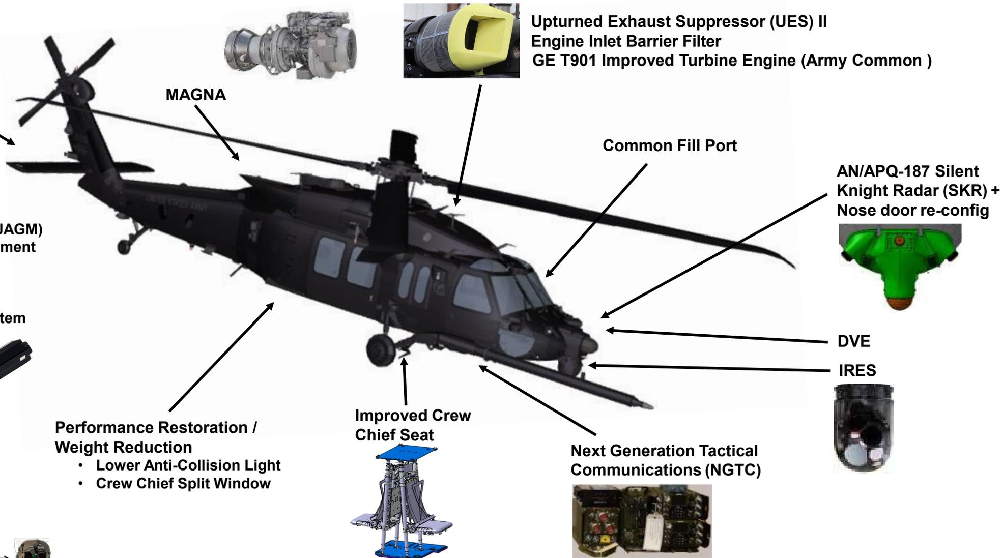
Modifications driven by restoration of payload and center of gravity
